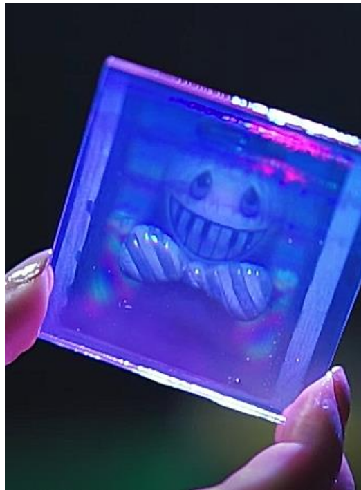
Hologram observed by transmission via halogen spot, after bleach. When the hologram is successful, this image will be very strong.
