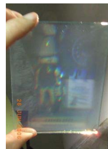
Fig. 4. When the plate is in wet state, the image can be observed by transmission.
